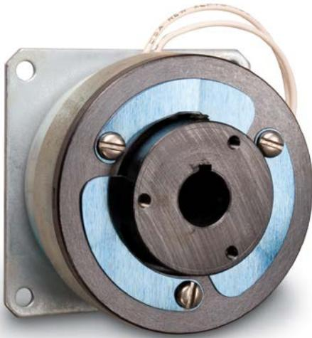
FB series power-on brakes are used to stop or hold a load that is coupled to the armature hub assembly. The armature hub is attached to the load shaft. The field assembly is mounted to a bulkhead that is perpendicular to the shaft.
