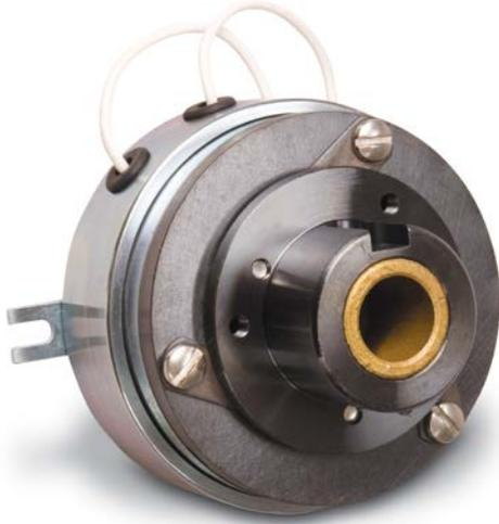
SL series power-on clutches are used to couple two parallel shafts. The armature hub assembly is mounted to the same shaft as the rotor assembly. The armature hub accommodates a pulley, gear, sprocket, etc., to transmit torque to the second shaft. The field assembly is mounted on the shaft and retained by a loose-fitting pin or bracket through the anti-rotation tab.
