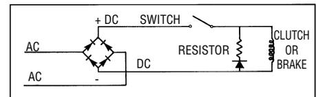
For faster release, use a zener diode with a rating two times the coil voltage.
