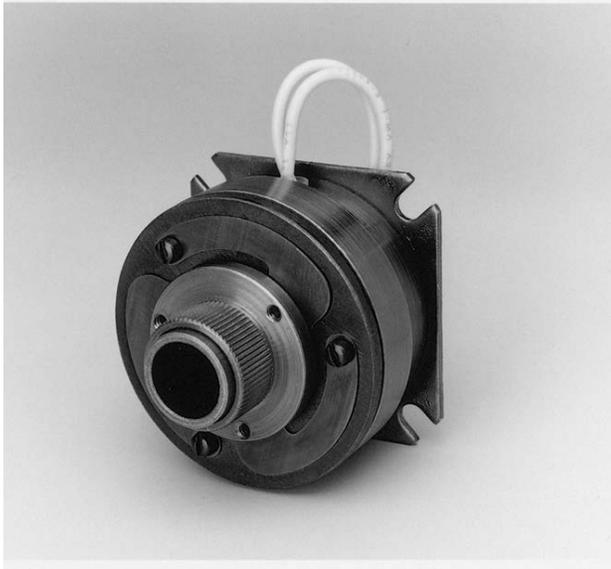
FL series power-on clutches are used to couple two parallel shafts. The armature hub assembly is mounted to the same shaft as the rotor assembly. The armature hub accommodates a pulley, gear, sprocket, etc., to transmit torque to the second shaft. The field assembly is mounted to a bulkhead that is perpendicular to the input shaft.
