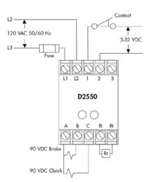
Wiring example for logic input 3-32 VDC
