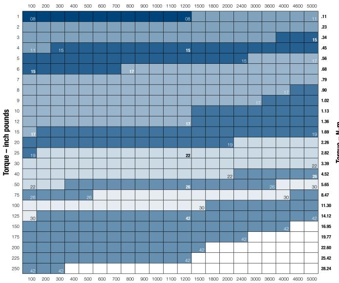
In addition to the solution steps on previous pages, the dynamic torque required may be calculated.
