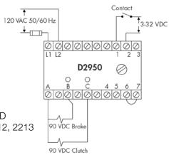
Wiring example for logic input 3-32 VDC
