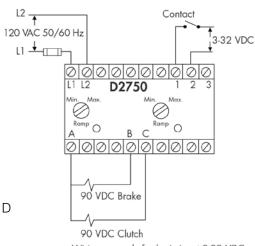
Wiring example for logic input 3-32 VDC
